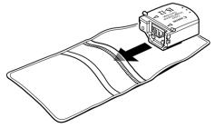
**6.** Remove the BJ Cartridge from the BJ Cartridge Container.
